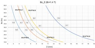
Figure 8: Field by magnet (different size and distance)
