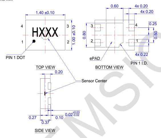
Figure 10: Mechanical package outline dimensions
