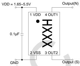
Figure 3: Connection diagram
