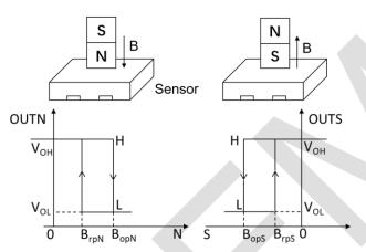
Figure 6: Output signals of OUTN and OUTS pins
