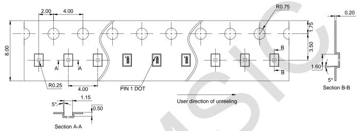
Figure 11: Carrier tape dimension and device orientation
