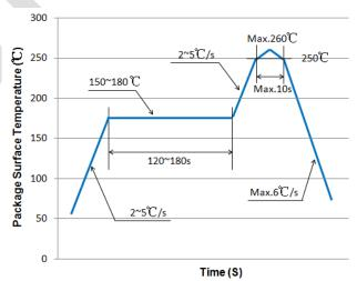
Figure 9: Recommended solder reflow profile
